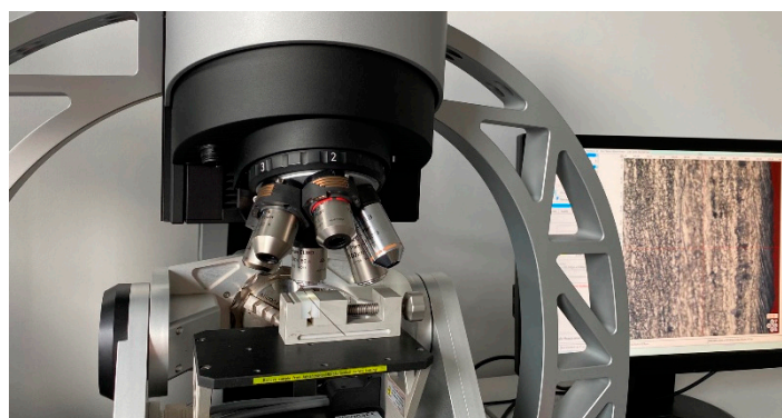
Figure 2. A focus variation microscope used for topography measurements with a wire in a holder.
