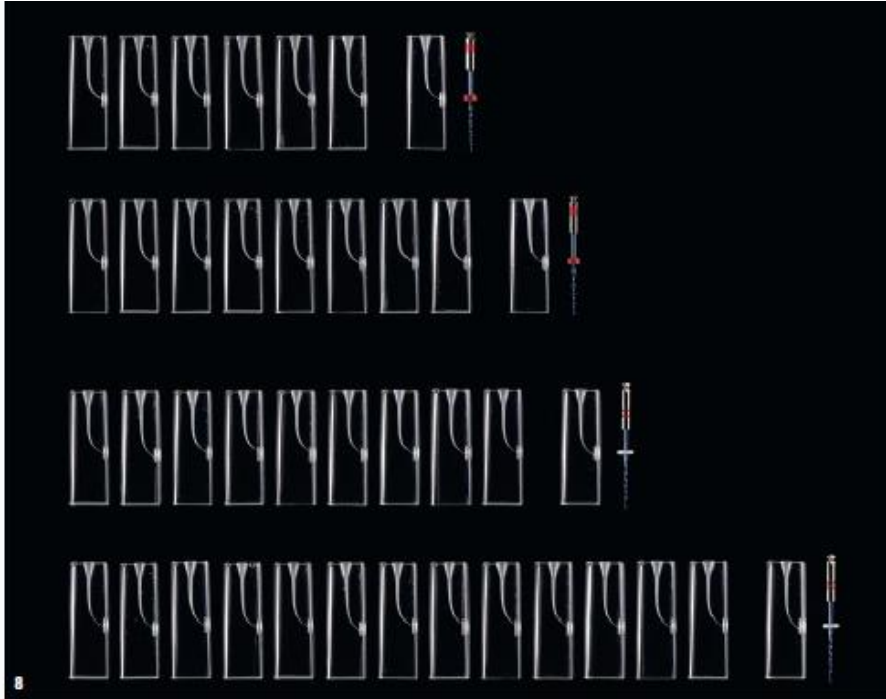
Fig. 8: First line (RECIPROC blue R25, continuous rotation): six blocks prepared without fracture, and the file fractured inside the seventh block. Second line (RECIPROC blue R25, reciprocation): eight blocks prepared without fracture, and the file fractured inside the ninth block. Third line (Endostar E3 Azure 25/06, continuous rotation): nine blocks prepared without fracture, and the file fractured inside the tenth block. Fourth line (Endostar E3 Azure 25/06, OTR reciprocation): thirteen blocks prepared without fracture, and the file fractured inside the fourteenth block.
