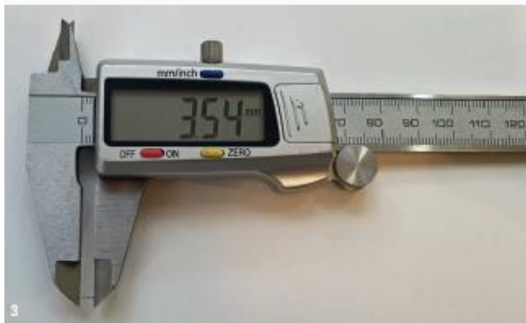
Fig. 3: Micro-caliper for measuring fractured instruments.
